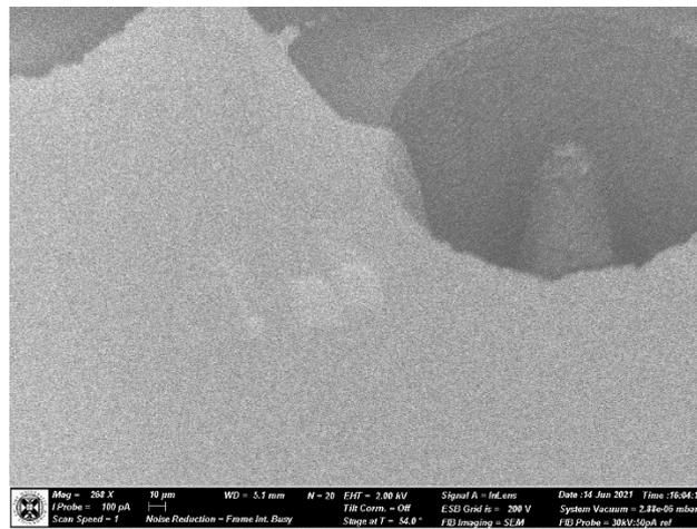
**Figure 2.** A zoomed-out image of the micropillar with three test FIB-SEM mills completed to the left of the micropillar. Note the zig-zag pattern showing the sample drifted during milling. This is a current outcome that continues to be troubleshooted.
