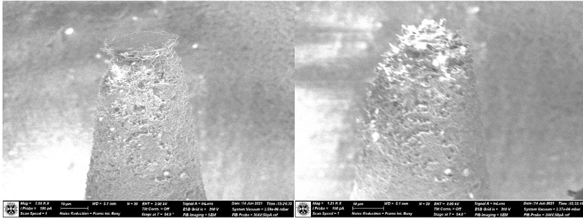
**Figure 1.** A micropillar on the CWC surface viewed in SEM before and after milling away the top layer. This was done to investigate the best way to SSV the aragonite crystals for 3D image reconstruction.
