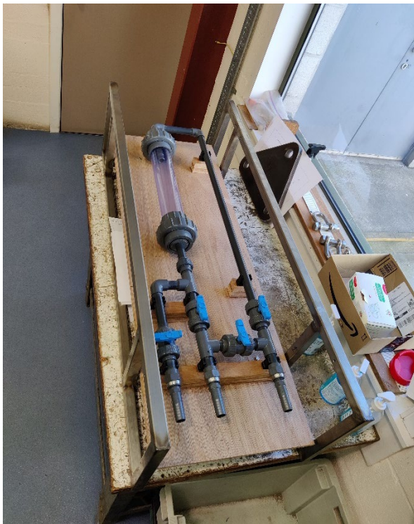
Figure 1. Image of the assembled ferry filter system.
