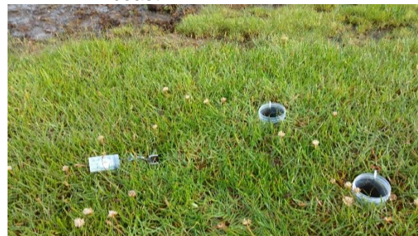
Fig. 2 Sediment traps and Hobo-G logger used as a Mini-Buoy to record inundation duration
