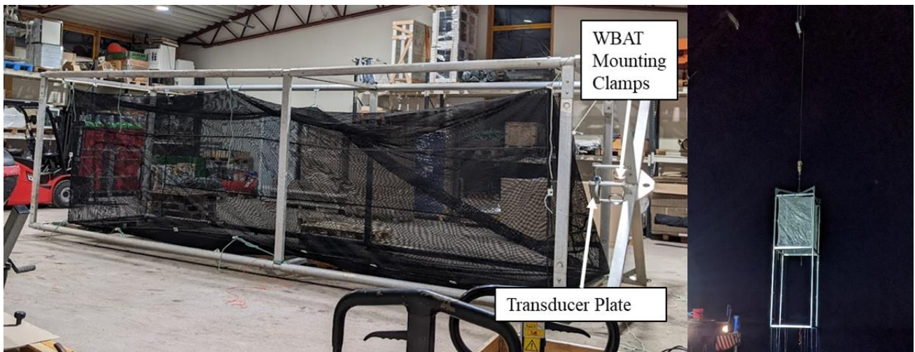
Figure 1. Left: Cage and fish net (mid-assembly). Right: Cage and zooplankton net in deployment orientation.
