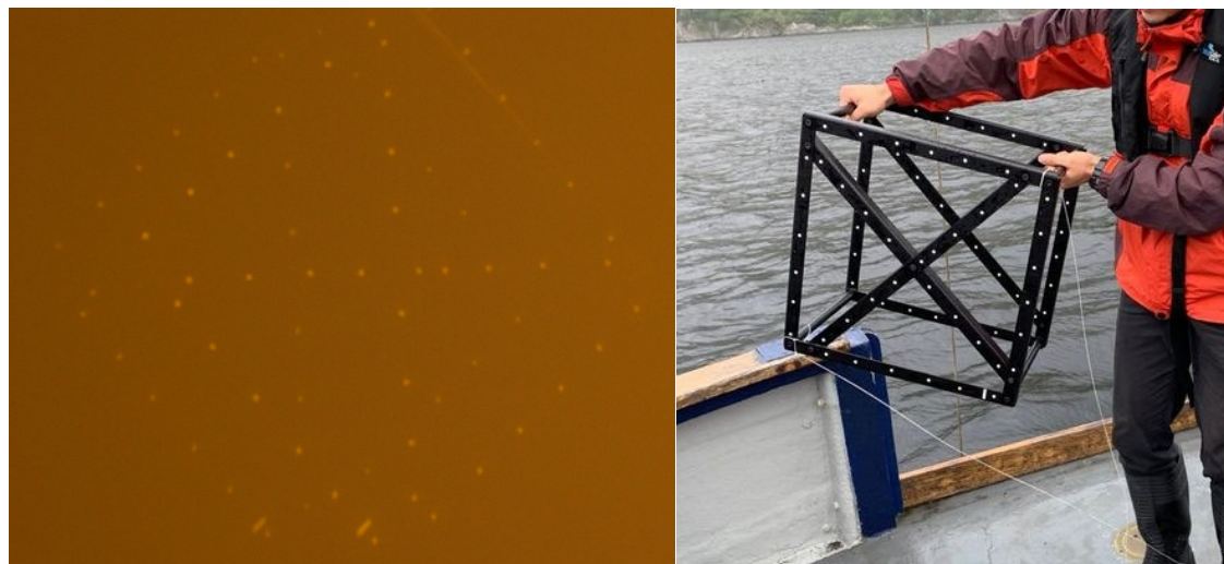
Figure 4. Calibration of stereo cameras. LEFT: Image of calibration cube near surface in murky water. RIGHT: Picture of calibration cube prior to deployment.
