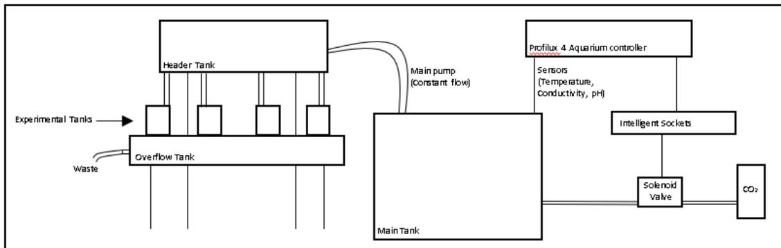
Figure 1: Experimental setup, GHF Profilux Aquarium Controller.
