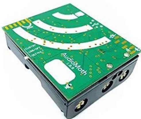
Figure 1A. An AudioMoth detector. The unit is ~ 5 x 4 x 2 cm in size. © Open Acoustic Devices.
