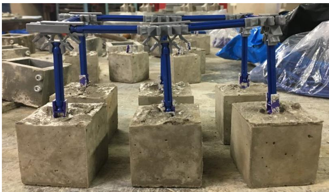
Figure 1: 6 trial concrete blocks attached to trial of K'NEX frame.
