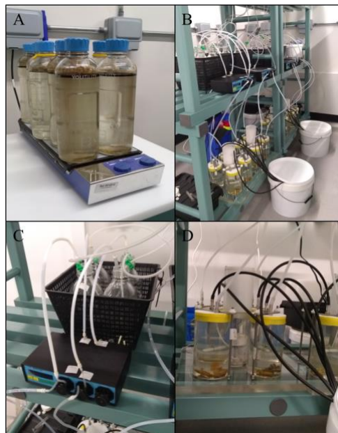
Figure 1 Experimental set-up (A) WAF and CEWAF preparations (B) Flow through set-up (C) Peristaltic pump (D) Individual incubation chamber
