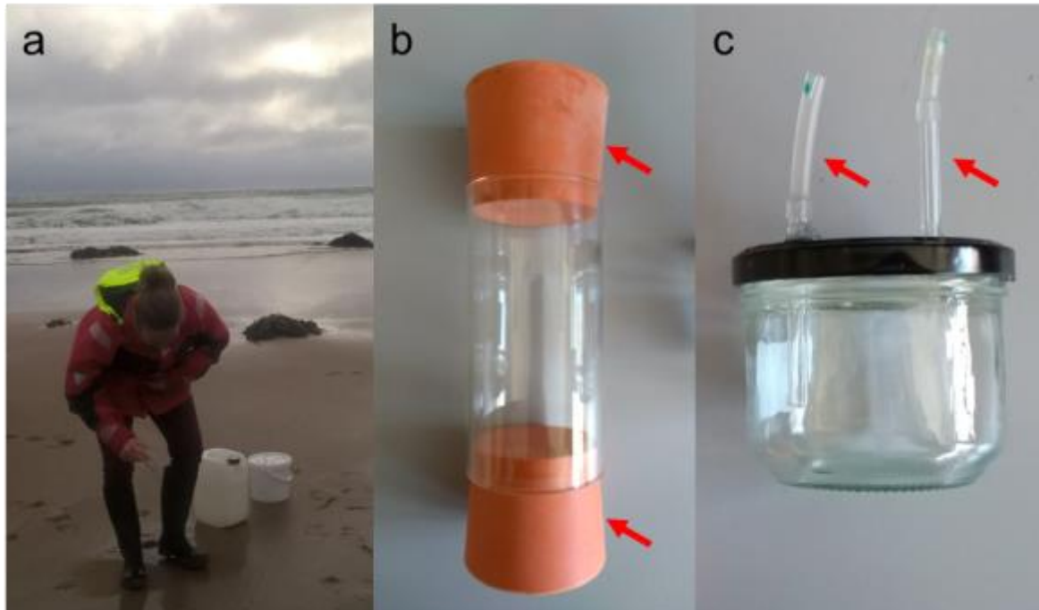
Figure 1 Sampling and incubation chambers used in this study. (a) Sampling of sediments and sponges took place at Coldingham Bay. (b) Glass corer used to sample sediments. The red arrows indicate the rubber bungs used to seal off the samples during collection. (c) Sponge incubation chamber used in this study. The red arrows indicate the inflow and outflow tubes.
