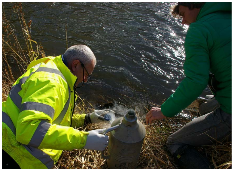
Figure 1: Taking sediment contact cores using liquid nitrogen from the bank of the River Eden beyond the tidal reach to assess potential sources to the saltmarsh carbon sink. Image: Clare Maynard
