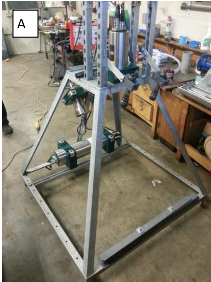
Figure 1. A) The benthic camera lander, prior to deployment. Borrom frame dimensions are ~1 x 1 m.
