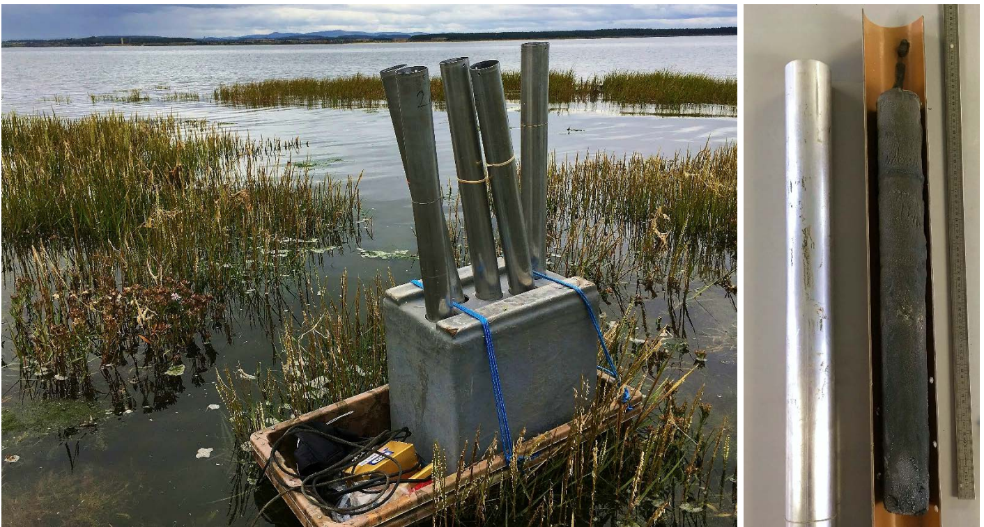
Figure 1. Left image showing series of core tubes and vibecore-mini head unit in the field ready for collection of sediment cores; Right image showing sediment core removed from core tube.
