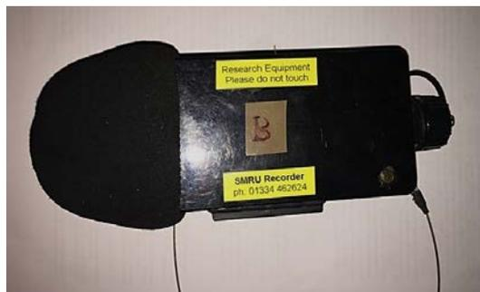
Fig. 1. Continuous sound recorder used for recordings of airborne sound at St Abb's Head, Berwickshire.
