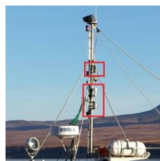
Electronic Monitoring System: Location of video cameras on mast
